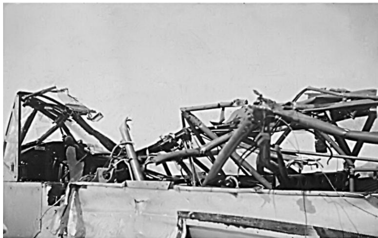
Right: The smashed cockpit on the lower plane after the plane on top was removed.
